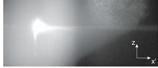
Fig. 5. CCD camera image of the trap in its low-population state in a plane parallel to the perturbing beam, showing the jet of atoms expelled from the trap.
